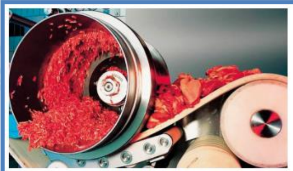
Picture 1: typical Deboning System
